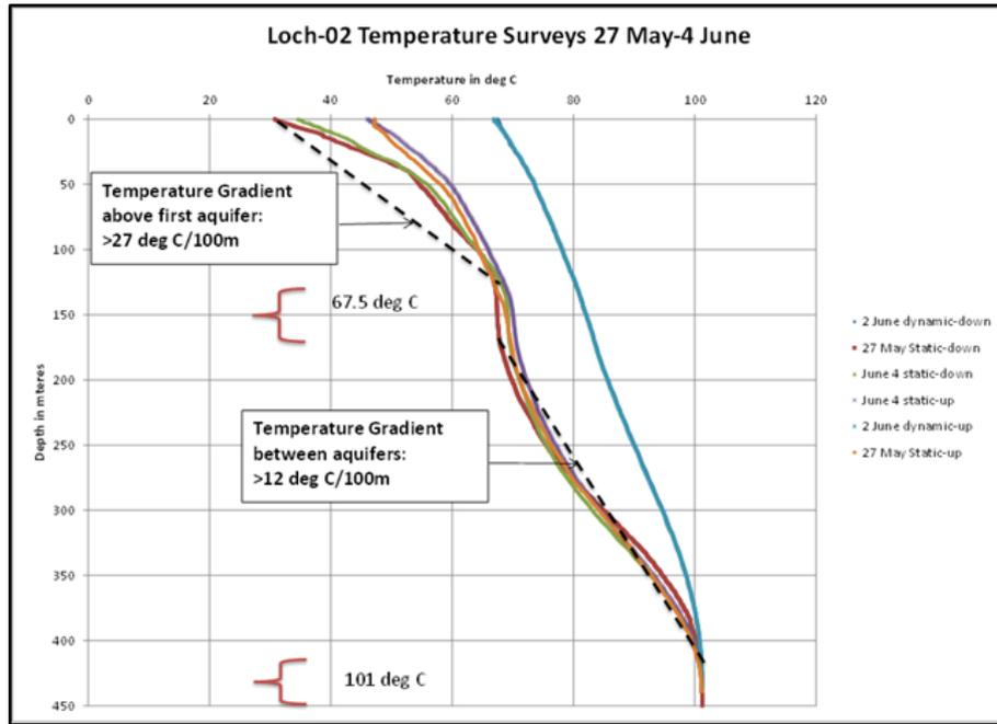
**Figure 5: Temperature gradient in Well LOCH 02**
