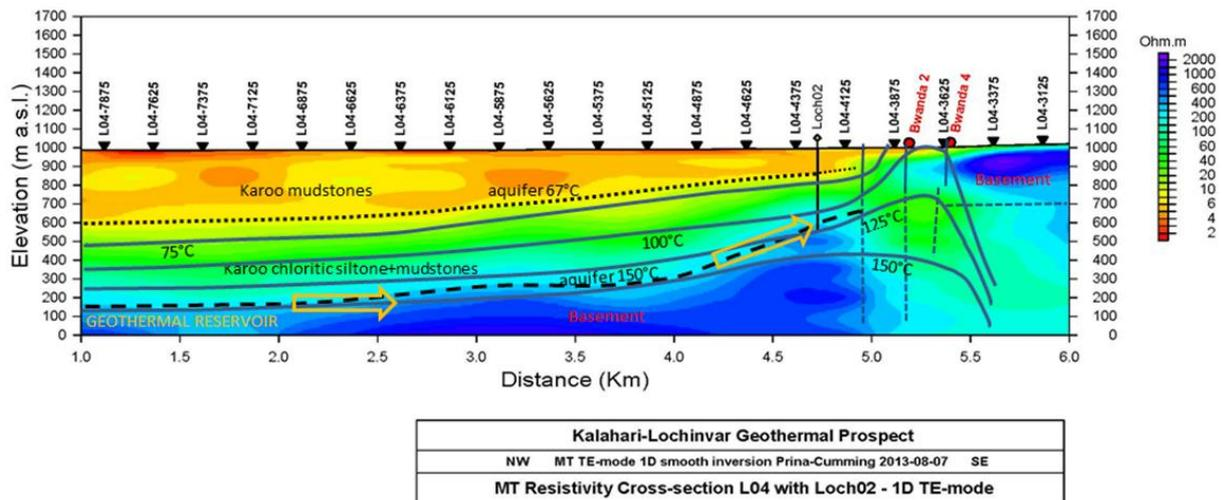
**Figure 4: MT Resistivity Cross Section through Well LOCH 02. The cross section is annotated with the key lithology, aquifers and temperature isobars as determined from Well LOCH 02, the total depth of which is 440m.**
