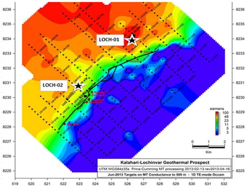
Figure 3: Bounding fault at surface, hot springs and Well locations on MT Conductance to 500m
